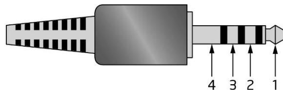
Figure 4. 4-Pin 3.5 mm (1/8 inch) Audio Jack Pin Out
